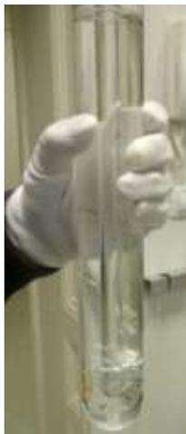
**Figure 2:** A water triple point cell (WTP)
