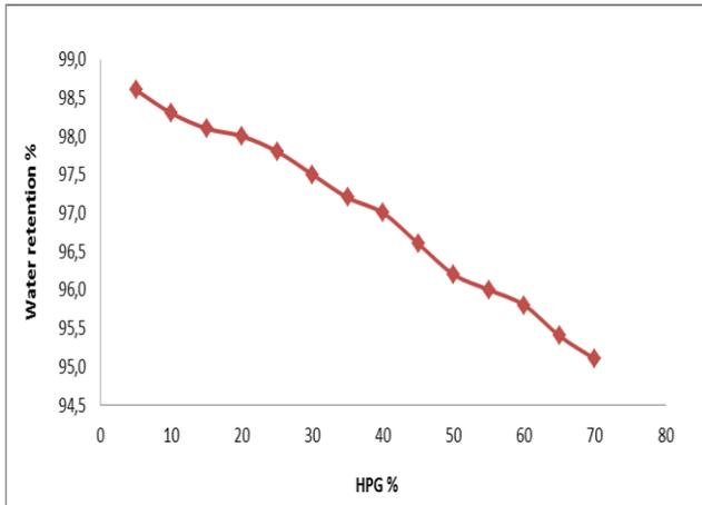
Figure 3: Water retention of freshly mixed cement based render-
