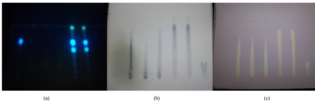
**Figure 1:** Thin layer chromatograms of bark extracts with different detection. (a) UV 365nm, (b) Folin-Ciocalteu reagent, (c) DPPH solution.
